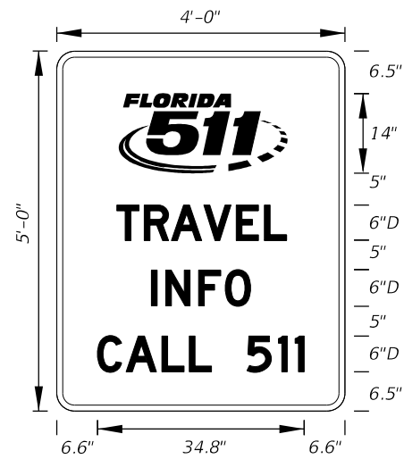
FTP-414-25 4'-0" X 5'-0" 3" Radii 1" Border 6" Series D Legend Blue Background White Legend and Border
