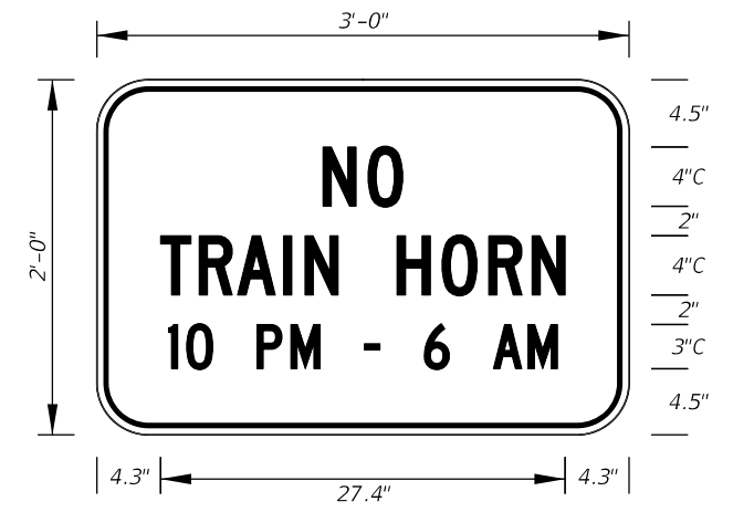
FTP-203-25 3'-0" X 2'-0" 1.5" Radii \frac{3}{4} " Border 4" and 3" Series C Legend Yellow Background Black Legend and Border
