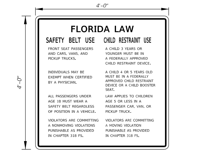
FTP-006-25 4'-0" X 4'-0" 1.5" Radii 0.4" Border 2.5" Series C Legend 2" Series C Legend 1.5" Series C Legend and White Background Black Legend and Border
