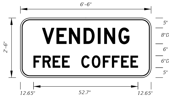
FTP-410-25 6'-6" X 2'-6" 3" Radii 3/4" Border 6" Series D Legend Blue Background White Legend and Border
