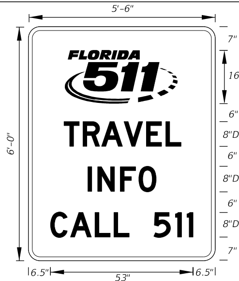
FTP-414A-25 5'-6" X 6'-0" 3" Radii 1" Border 8" Series D Legend Blue Background White Legend and Border
