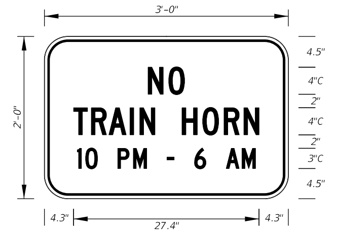
FTP-203-25 3'-0" X 2'-0" 1.5" Radii 3/4" Border 4" and 3" Series C Legend Yellow Background Black Legend and Border
