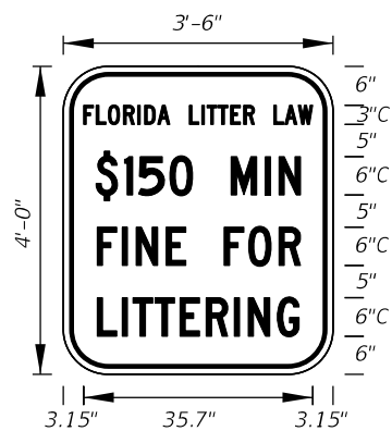
FTP-015A-25 3'-6" X 4'-0" 1.5" Radii 3/4" Border 3" and 6" Series C Legend White Background Black Legend and Border
