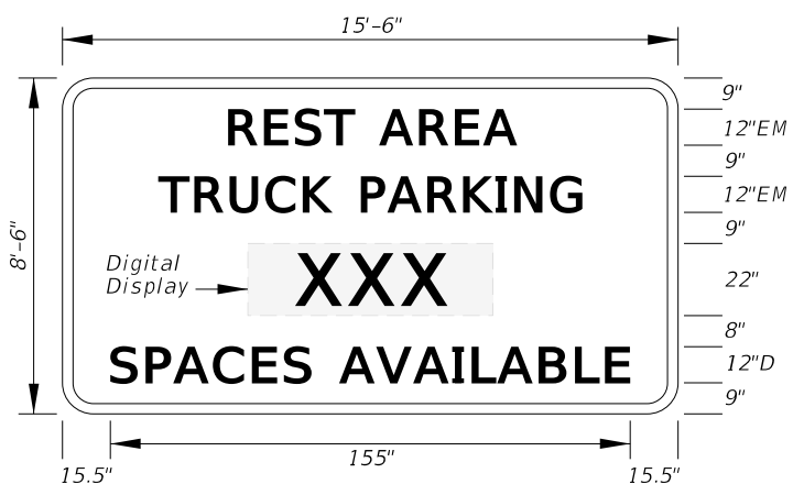
FTP-406-25 15'-6" X 8'-6" 12" Radii 2" Border 12" Series EM Legend 12" Series D Legend Blue Background White Legend and Border
