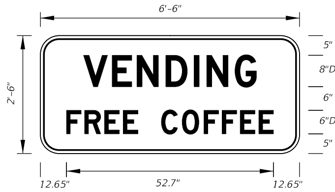
FTP-410-25 6'-6" X 2'-6" 3" Radii 3/4" Border 8" and 6" Series D Legend Blue Background White Legend and Border
