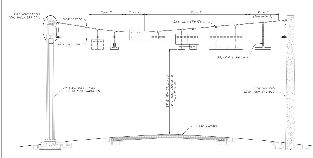
TYPICAL INSTALLATIONS FOR SIGN PANEL(S) MOUNTED ON SPAN WIRE:
