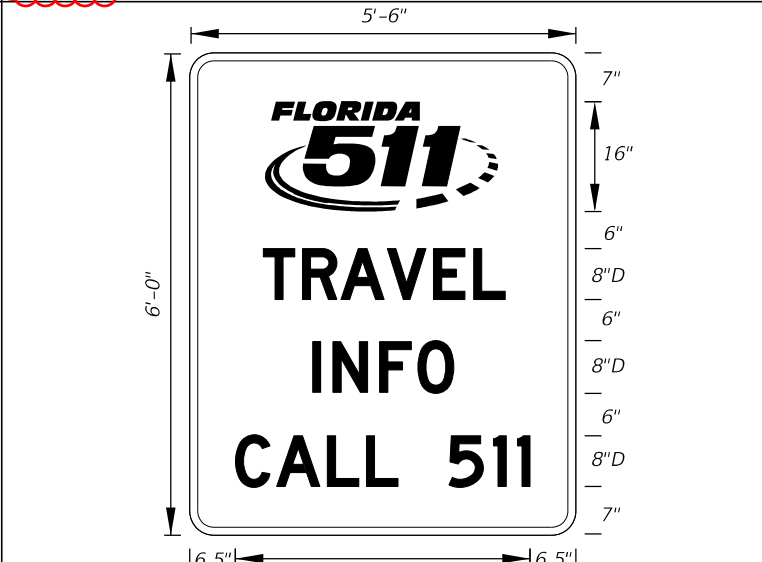
FTP-414A-25 5'-6" X 6'-0" 3" Radii 1" Border 8" Series D Legend Blue Background White Legend and Border
