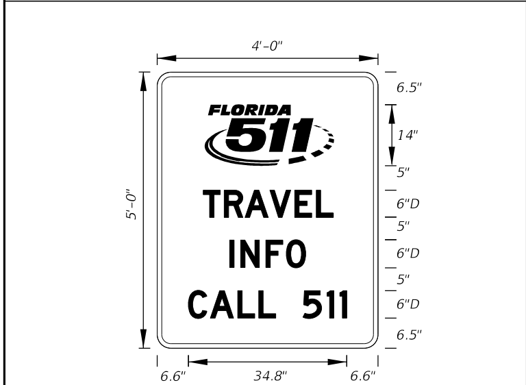
FTP-414-25 4'-0" X 5'-0" 3" Radii 1" Border 6" Series D Legend Blue Background White Legend and Border
