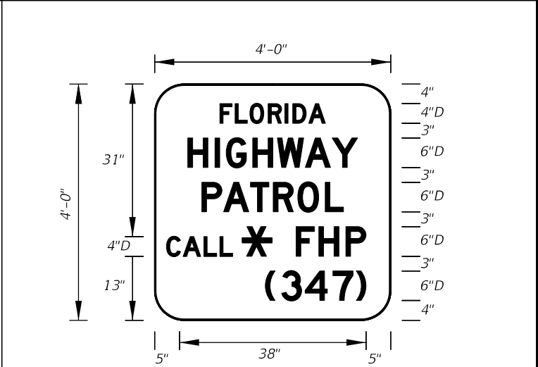
FTP-413-25 4'-0" X 4'-0" 3" Radii 1" Border 4" and 6" Series D Legend Blue Background White Legend and Border
