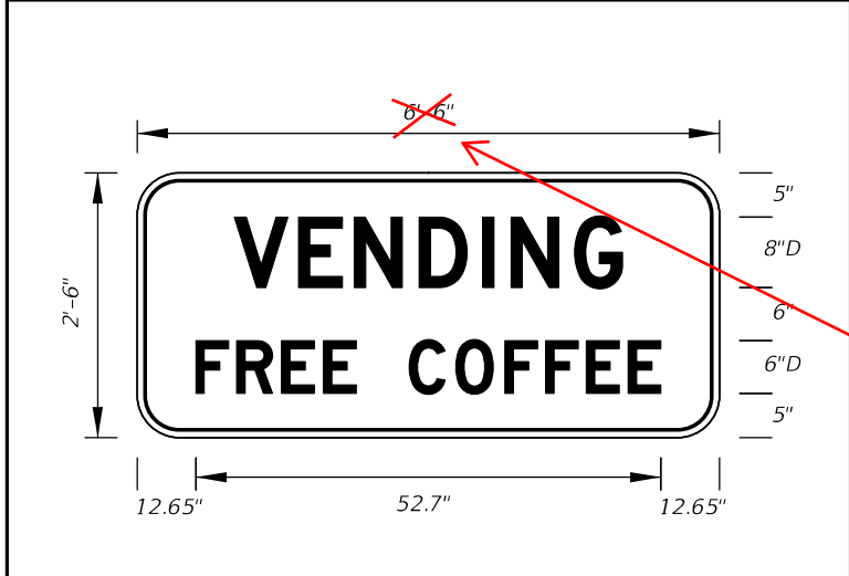
FTP-410-25 6'-6" X 2'-6" 3" Radii ¾" Border 8" and 6" Series D Legend Blue Background White Legend and Border
