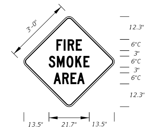
FTP-72-06 3' X 3' 2" Radii 3/4" Border 6" Series C Legend Yellow Background Black Legend and Border
