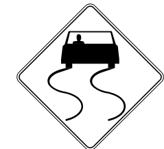
W8-5 SLIPPERY WHEN WET SIGN See Note 11
