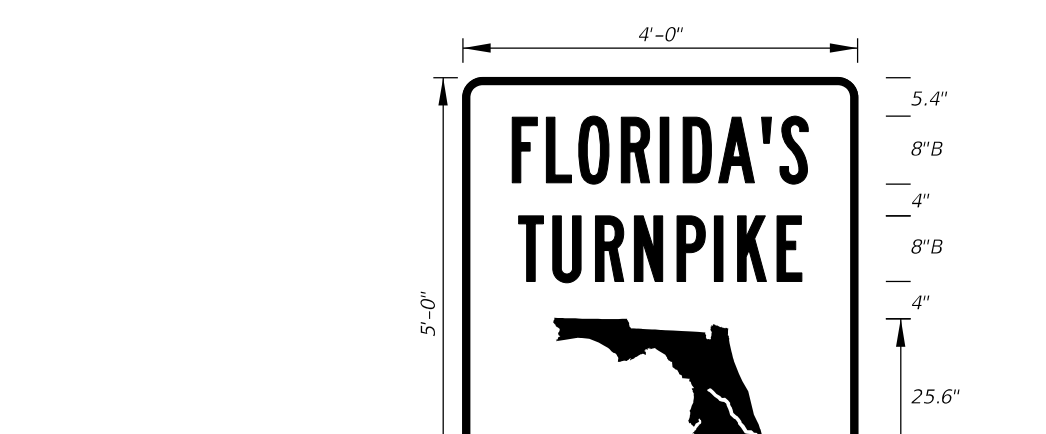
FTP-18-10 4'-0" X 5'-0" 3" Radii 1 1/4" Border 8" Series B Legend Green Background White Legend, Border, and Florida Symbol
