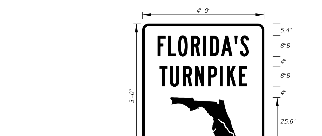
FTP-18-10 4'-0" X 5'-0" 3" Radii 1 1/4" Border 8" Series B Legend Green Background White Legend, Border, and Florida Symbol
