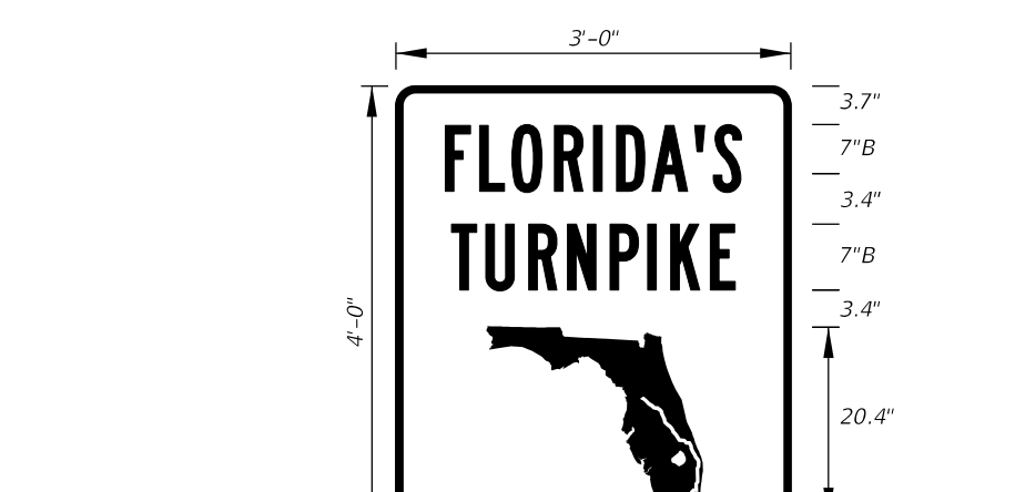
FTP-17-10 3'-0" X 4'-0" 1.5" Radii 3/4" Border 7" Series B Legend Green Background White Legend, Border, and Florida Symbol
