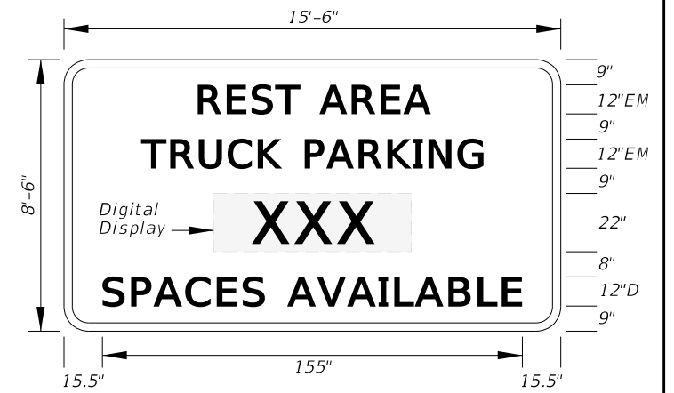
FTP-87-21 15'-6" X 8'-6" 12" Radii 2" Border Series D Legend Series EM Legend Blue Background White Legend and Border
