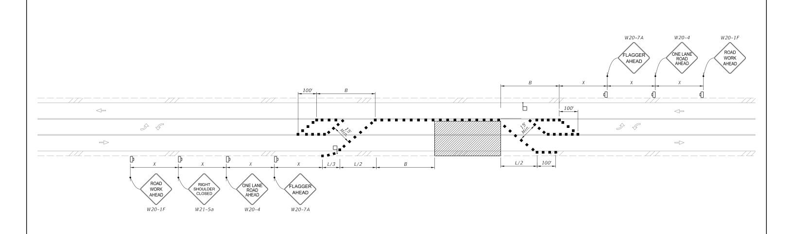
= TEMPORARY TWO-WAY LEFT-TURN LANE CLOSURE, TWO-LANE, TWO-WAY ROADWAY, WORK WITHIN THE =TRAVELED WAY WITH LANE CLOSURES OF 24 HRS OR LESS AND WORK ZONE SPEED OF 45 MPH OR LESS
