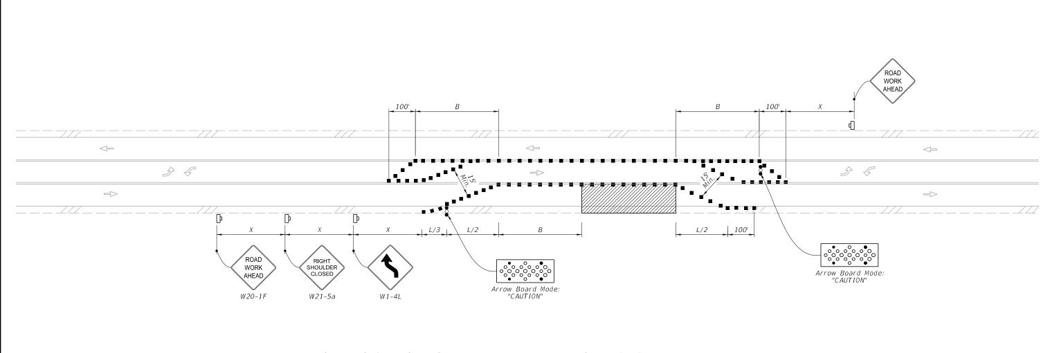
$\equiv$  TEMPORARY SHIFT TO TWO-WAY LEFT-TURN LANE, WORK WITHIN THE TRAVELED WAY = WITH LANE CLOSURES OF 24 HRS OR LESS AND WORK ZONE SPEED OF 45 MPH OR LESS
