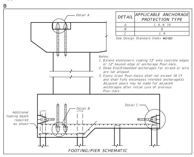
Prepare tendon Mockups and associated details and include them in the plans for use in combination with the filler injection demonstrations required by *Specifications*Section 462-7. Mockups are not required for grouted transverse tendons in the top slabs of box girders and for vertical bar tendons in the webs or diaphragms of box girders.
