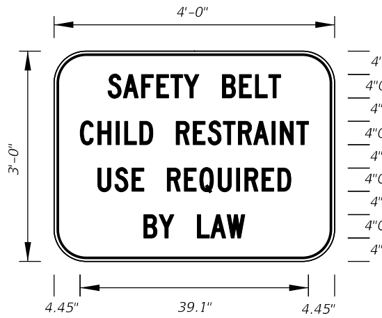
FTP-45-06 4' X 3' 5" Radii 3/4" Border 4" Series C Legend White Background Black Legend and Border
