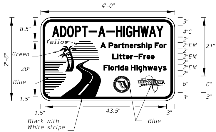
FTP-42-06 4' X 2'-6" 3" Radii Top 4" Series C Legend Bottom 2" Series EM Legend White Background Blue Legend and Border
