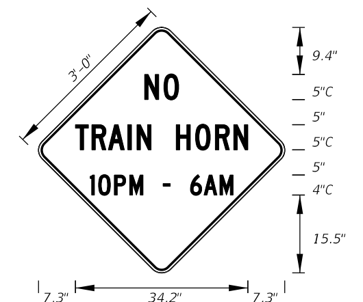
FTP-62-06 3' X 3' 2" Radii 3/4" Border 4" and 5" Series C Legend Yellow Background Black Legend and Border
