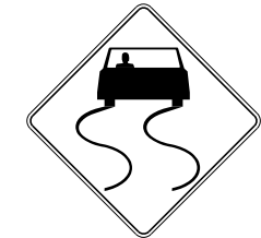
W8-5 SLIPPERY WHEN WET SIGN See Note 11
