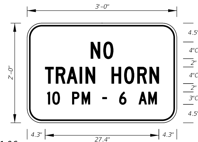
FTP-61-06 3' X 2' 3" Radii 3/4" Border 4" and 3" Series C Legend Yellow Background Black Legend and Border
