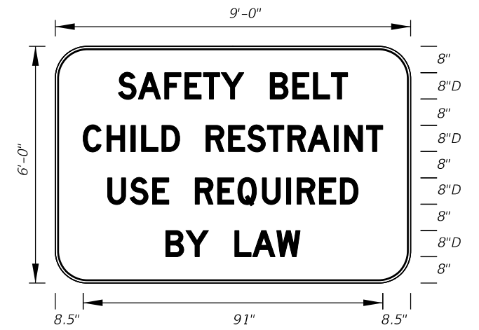
FTP-44-06 9' X 6' 9" Radii 3/4" Border 8" Series D Legend White Background Black Legend and Border
