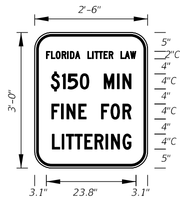
FTP-41-21 2'-6" X 3' 4" Radii 3/4" Border 2" and 4" Series C Legend White Background Black Legend and Border
