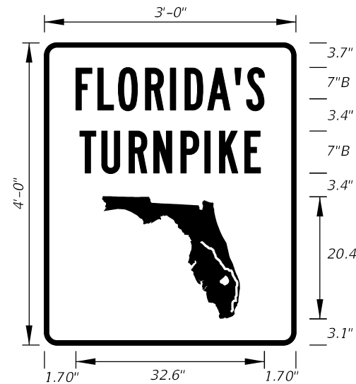
FTP-17-10 3'-0" X 4'-0" 1.5" Radii 3/4" Border 7" Series B Legend Green Background White Legend, Border, and Florida Symbol
