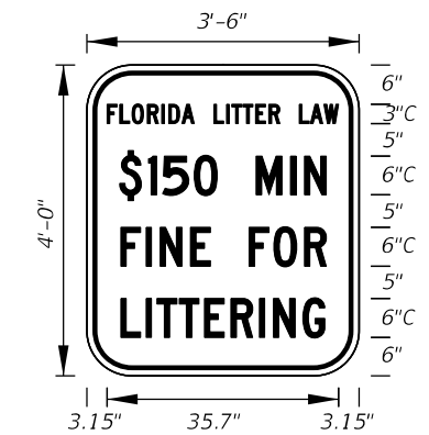
FTP-40-21 3'-6" X 4' 6" Radii 3/4" Border 3" and 6" Series C Legend White Background Black Legend and Border
