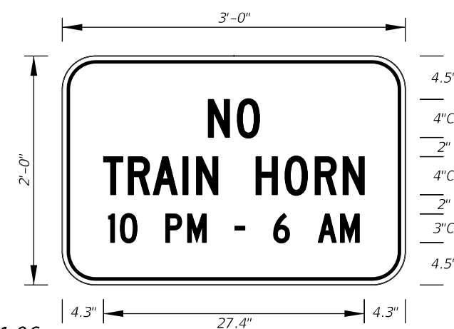
FTP-61-06 3' X 2' 3" Radii 3/4" Border 4" and 3" Series C Legend Yellow Background Black Legend and Border
