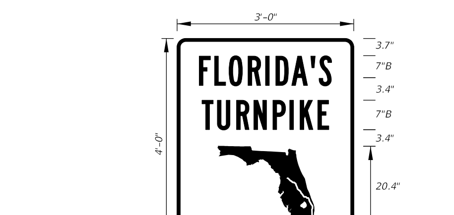
FTP-17-10 3'-0" X 4'-0" 1.5" Radii 3/4" Border 7" Series B Legend Green Background White Legend, Border, and Florida Symbol
