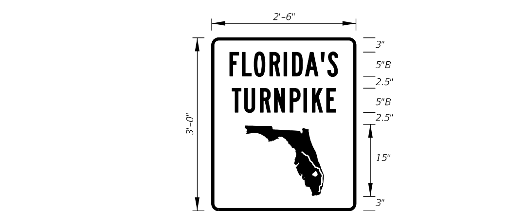
FTP-16-10 2'-6" X 3'-0" 1.5" Radii 3/4" Border 5" Series B Legend Green Background White Legend, Border, and Florida Symbol
