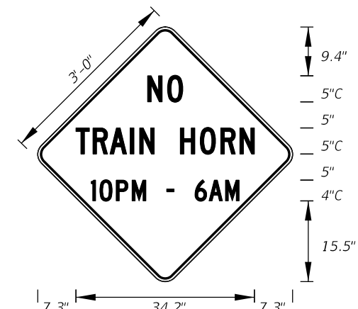
FTP-62-06 3' X 3' 2" Radii 3/4" Border 4" and 5" Series C Legend Yellow Background Black Legend and Border
