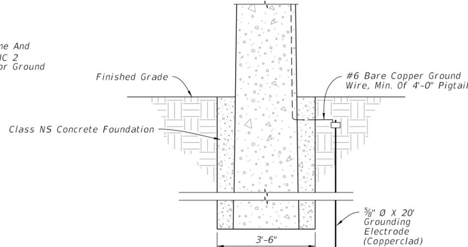
PRESTRESSED CONCRETE STRAIN POLE
