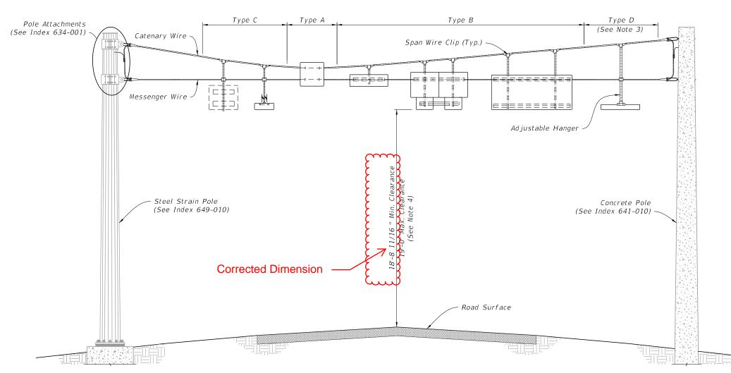
TYPICAL INSTALLATIONS FOR SIGN PANEL(S) MOUNTED ON SPAN WIRE =
