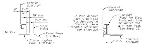
TYPICAL GRADING & PAVT. PLACEMENT DETAIL (See Note 2)
