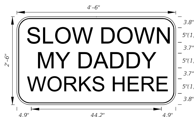
MOT-12R-06 2' X 1' 2" Radii 3/4" Border 2" Series B Legend White Background Black Legend and Border
