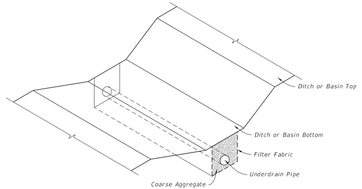
**UNDERDRAIN TYPE I, II, AND III ASSEMBLY**
