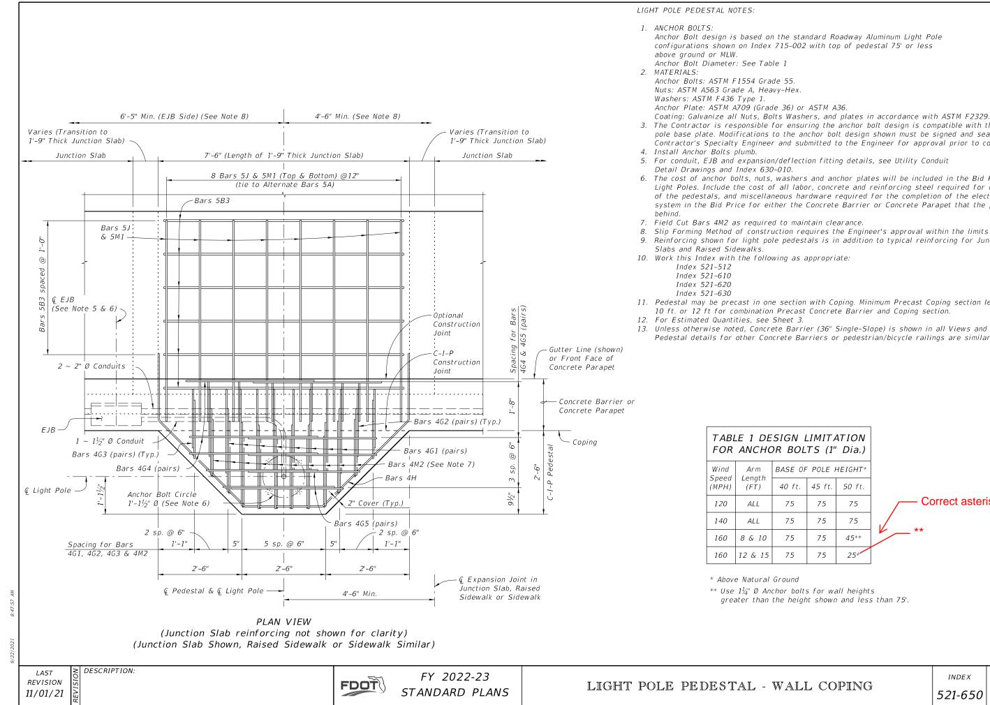
3. The Contractor is responsible for ensuring the anchor bolt design is compatible with the light pole base plate. Modifications to the anchor bolt design shown must be signed and sealed by the Contractor's Specialty Engineer and submitted to the Engineer for approval prior to construction.
