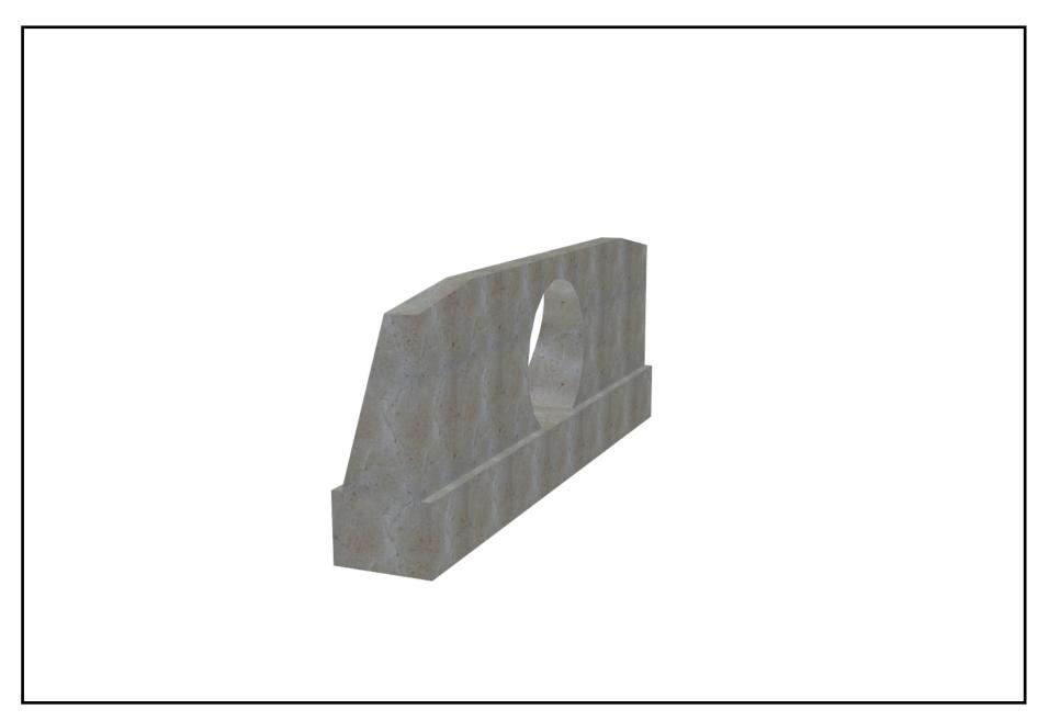
INDEX 430-030 Straight Concrete Endwalls Single and Multiple Pipe (Single 54" With O Degree Skew Pipe Shown)
