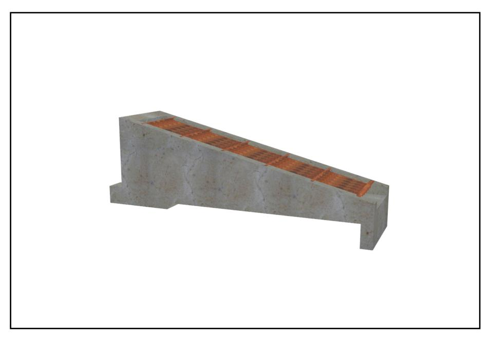
INDEX 430-010 U-Type Concrete Endwalls With Grates - 15" to 30" Pipe (30" Pipe With Grate Shown)
