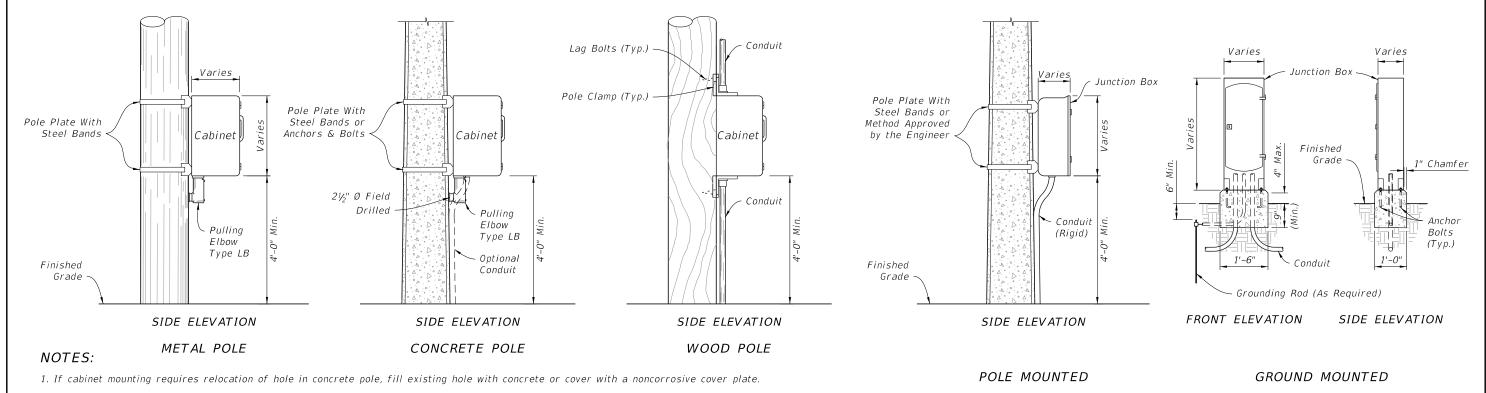
2. Liquidtight flexible conduit is approved for use from the electrical disconnect to the cabinet when both are installed on the same pole.
