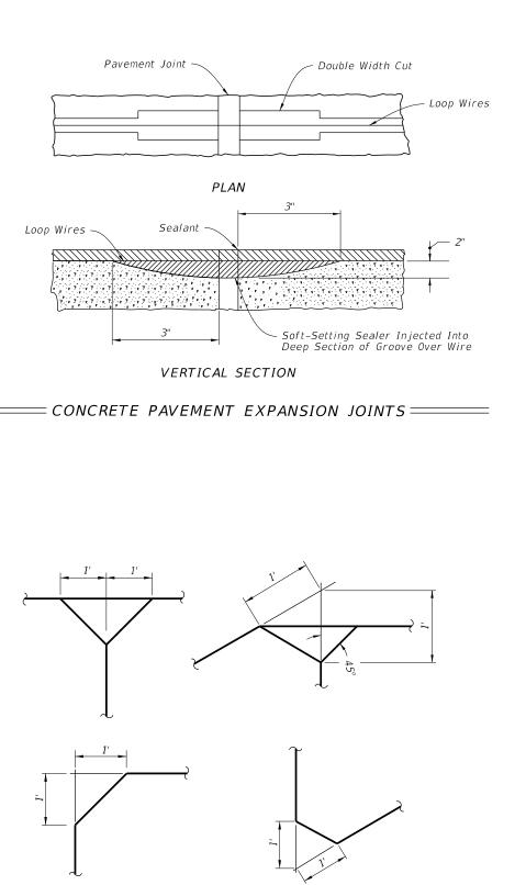
\_\_\_\_ LOOP CORNER AND LEAD-IN DETAILS \_\_\_\_\_\_
