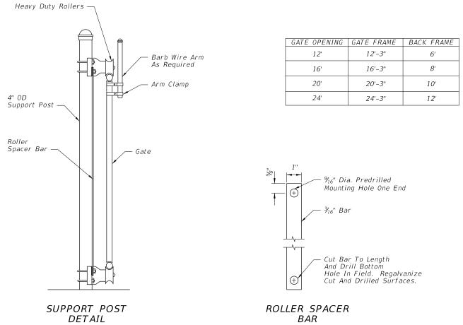
1. Extruded, rolled or formed components that provide equal strength and stability may be used in lieu of the pipe components shown; and, internal rollers may be used in lieu of the external roller units shown.
