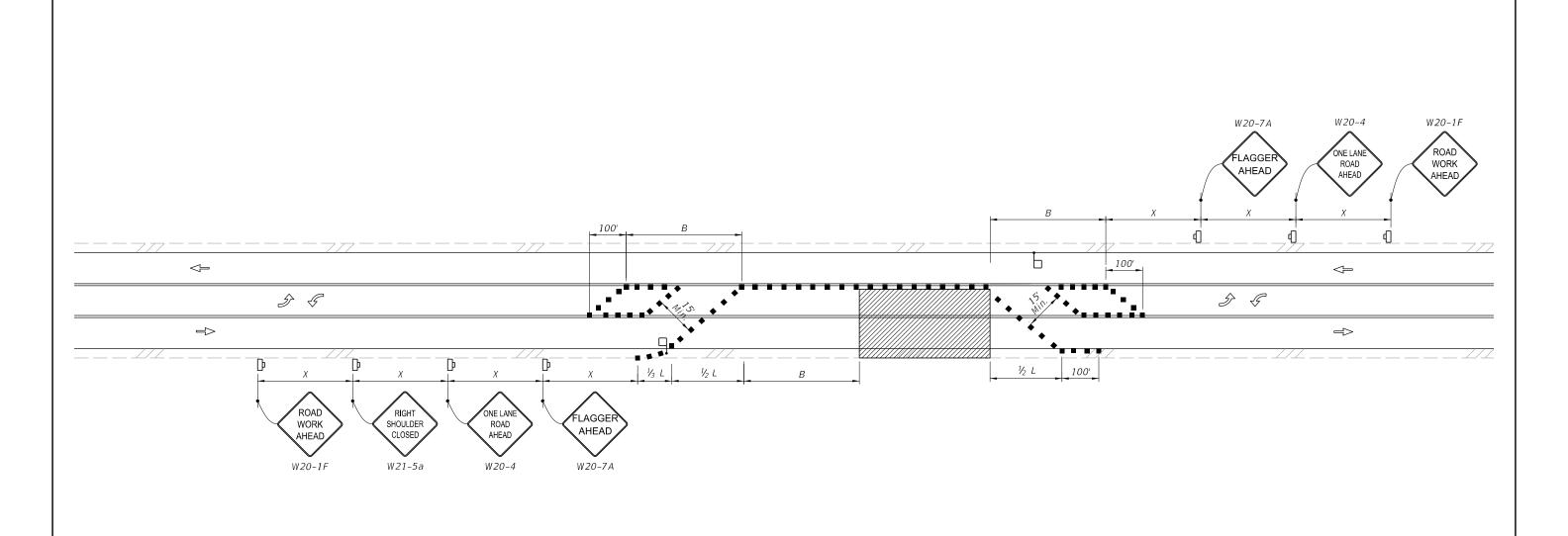
= TEMPORARY TWO-WAY LEFT-TURN LANE CLOSURE, TWO-LANE, TWO-WAY ROADWAY, WORK WITHIN THE =TRAVELED WAY WITH LANE CLOSURES OF 24 HRS OR LESS AND WORK ZONE SPEED OF 45 MPH OR LESS
