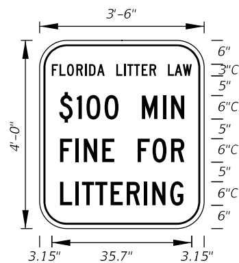
FTP-40-06 3'-6" X 4' 6" Radii 3/4" Border 3" and 6" Series C Legend White Background Black Legend and Border
