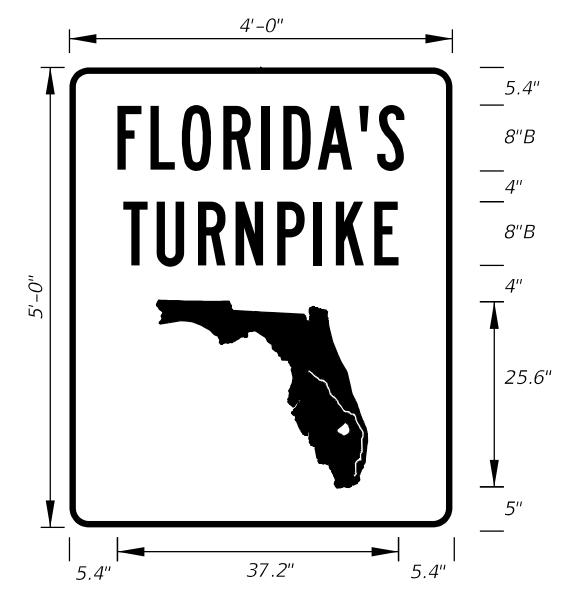
FTP-18-10 4'-0" X 5'-0" 3" Radii 1 1/4" Border 8" Series B Legend Green Background White Legend, Border, and Florida Symbol
