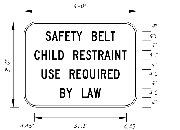
FTP-45-06 4' X 3' 5" Radii 3/4" Border 4" Series C Legend White Background Black Legend and Border
