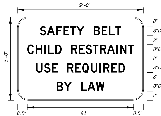
FTP-44-06 9' X 6' 9" Radii 3/4" Border 8" Series D Legend White Background Black Legend and Border
