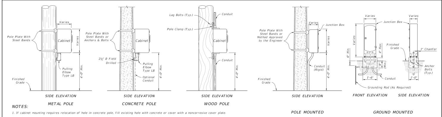
2. Liquidtight flexible conduit is approved for use from the electrical disconnect to the cabinet when both are installed on the same pole.
