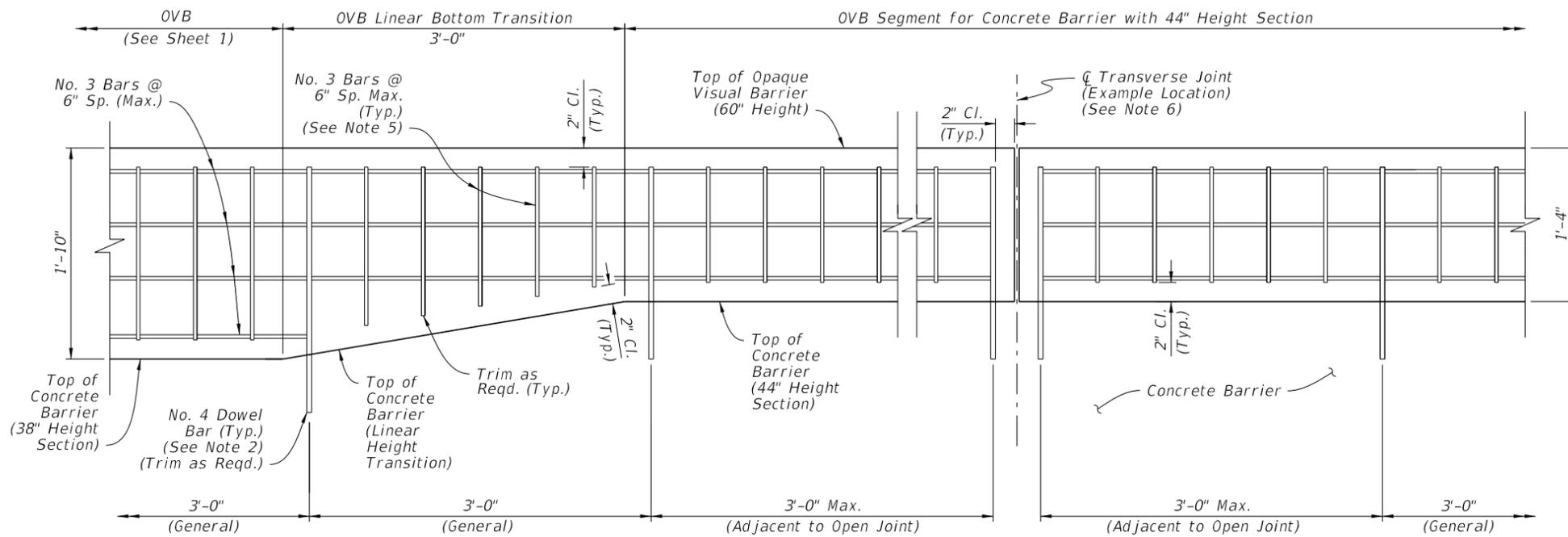
**ELEVATION VIEW 'B' - OVB SEGMENT FOR CONCRETE BARRIER WITH 44" HEIGHT SECTION (OVB LINEAR BOTTOM TRANSITION SHOWN, REVERSE DIRECTION SIMILAR BY OPPOSITE HAND)**
