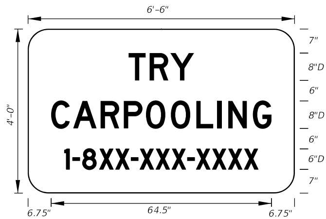
FTP-56-06 6'-6" X 4' 6" Radii 3/4" Border 8" and 6" Series D Legend Blue Background White Legend and Border Design Project Manager or Transit Administrator will supply correct 1-8XX number.
