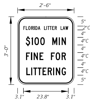
FTP-41-06 2'-6" X 3' 4" Radii 3/4" Border 2" and 4" Series C Legend White Background Black Legend and Border
