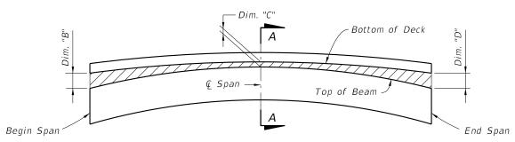
BUILD-UP DIAGRAM FOR CREST VERTICAL CURVE SPANS - CONTROL AT Q SPAN (ALONG G FLANGE) (CASE 3)
