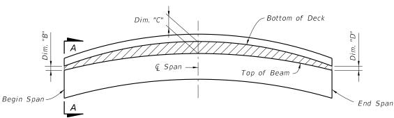
BUILD-UP DIAGRAM FOR CREST VERTICAL CURVE SPANS - CONTROL AT BEGIN OR END SPAN (ALONG G FLANGE) (CASE 4)
