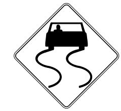
W8-5 SLIPPERY WHEN WET SIGN See Note 11
