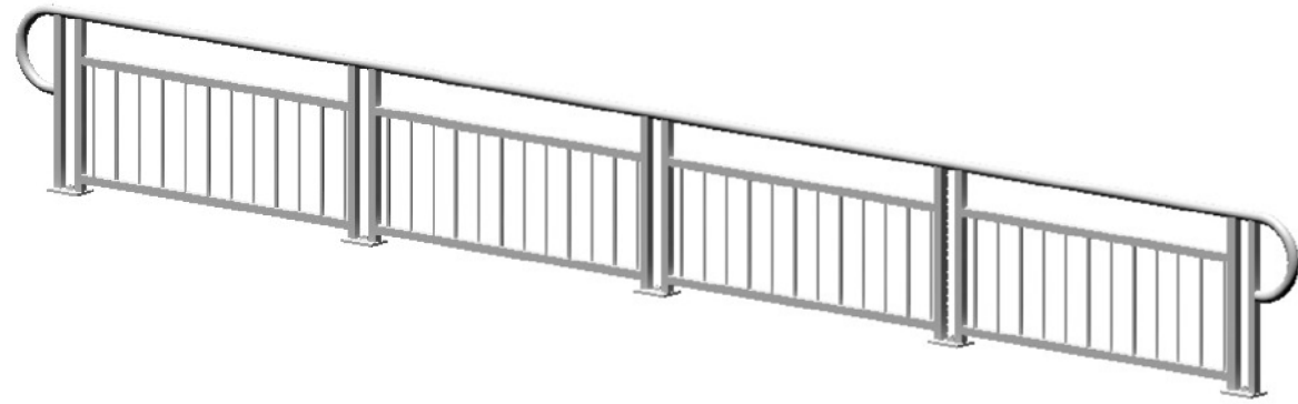
3D VIEW OF RAILING WITH TYPE 1 - PICKET INFILL PANEL (42" Height shown, 48" Height Similar)
