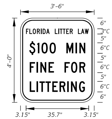
FTP-40-06 3'-6" X 4' 6" Radii 3/4" Border 3" and 6" Series C Legend White Background Black Legend and Border
