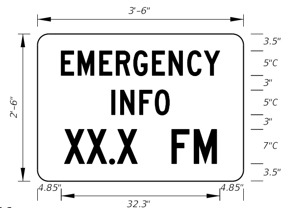
FTP-70-06 3'-6" X 2'-6" 2.25" Radii 3/4" Border 5" Series C and 7" Series C Legend Blue Background White Legend and Border
