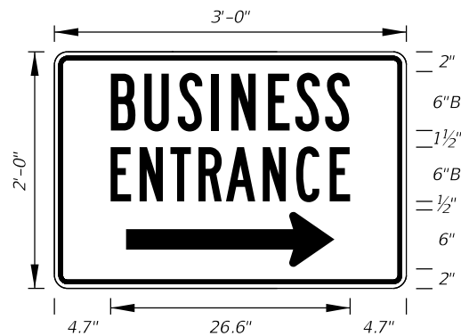
MOT-11-06 3' X 2' 2" Radii 3/4" Border 6" Series B Legend Blue Background White Legend and Border
