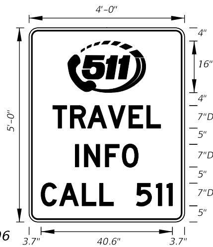
FTP-60-06 3' X 2' 3" Radii 4" and 3" Series C Legend Blue Background White Legend and Border Design Project Manager or Transit Administrator will supply correct 1-8XX number.
