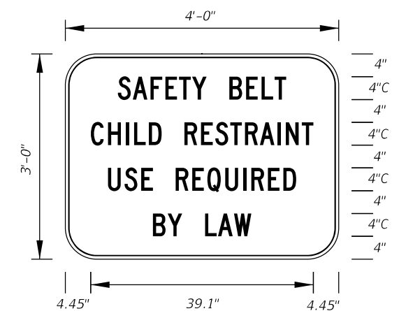
FTP-45-06 4' X 3' 5" Radii 3/4" Border 4" Series C Legend White Background Black Legend and Border
