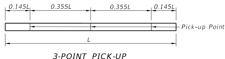
PILE PICK-UP DETAILS
