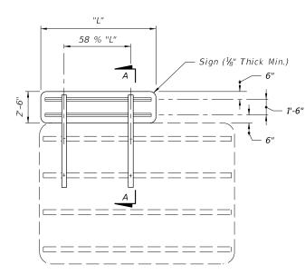
NOTE: Exit numbering panel shall be located to the right side for right exit and to the left for left exit.
