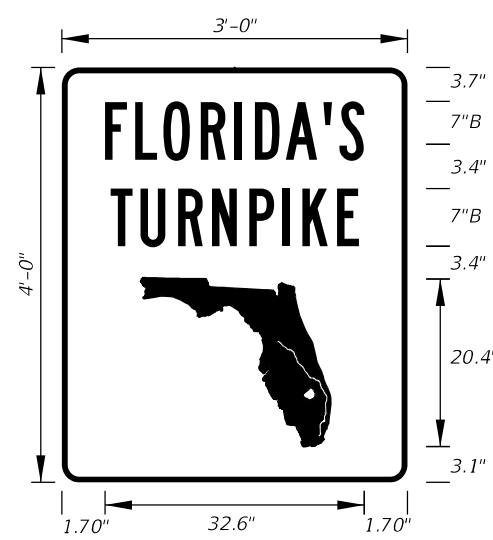
FTP-17-10 3'-0" X 4'-0" 1.5" Radii 3/4" Border 7" Series B Legend Green Background White Legend, Border, and Florida Symbol
