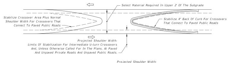
Limits Of Stabilization For Intermediate U-turn Crossovers And, Unless Otherwise Called For In The Plans, At Paved And Unpaved Private Roads And Unpaved Public Roads. Stabilize Crossover Area Plus Normal Stabilize Crossover Area Plus Normal Shoulder Width For Crossovers That Shoulder Width For Crossovers That Connect To Paved Public Roads Connect To Paved Public Roads  $\Rightarrow$ Select Material Required In Upper 24" Of The Subgrade -
