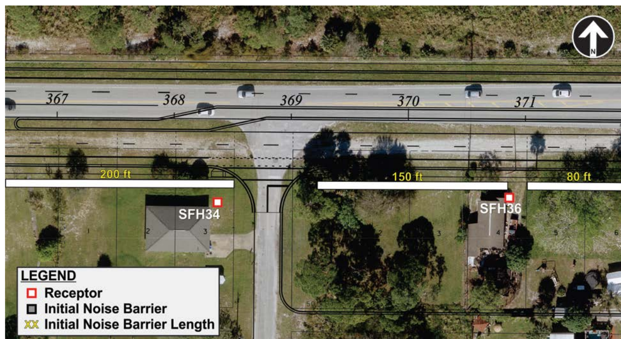
Figure 6-1 Noise Barrier Analysis
