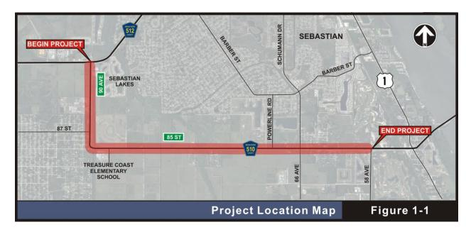
The existing right-of-way along the corridor varies from approximately 80 to 160 feet wide. CR-510 is owned and maintained by Indian River County and is functionally classified as an urban principal arterial. The proposed project will provide additional capacity to meet the future traffic needs resulting from projected population and employment growth within the projected area, expected as a result of various proposed residential developments.
