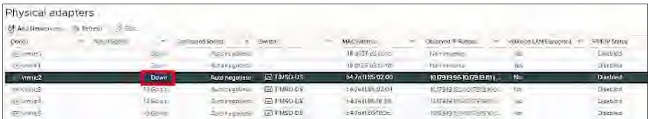
Figure 144. Confirm that the Port is Down
